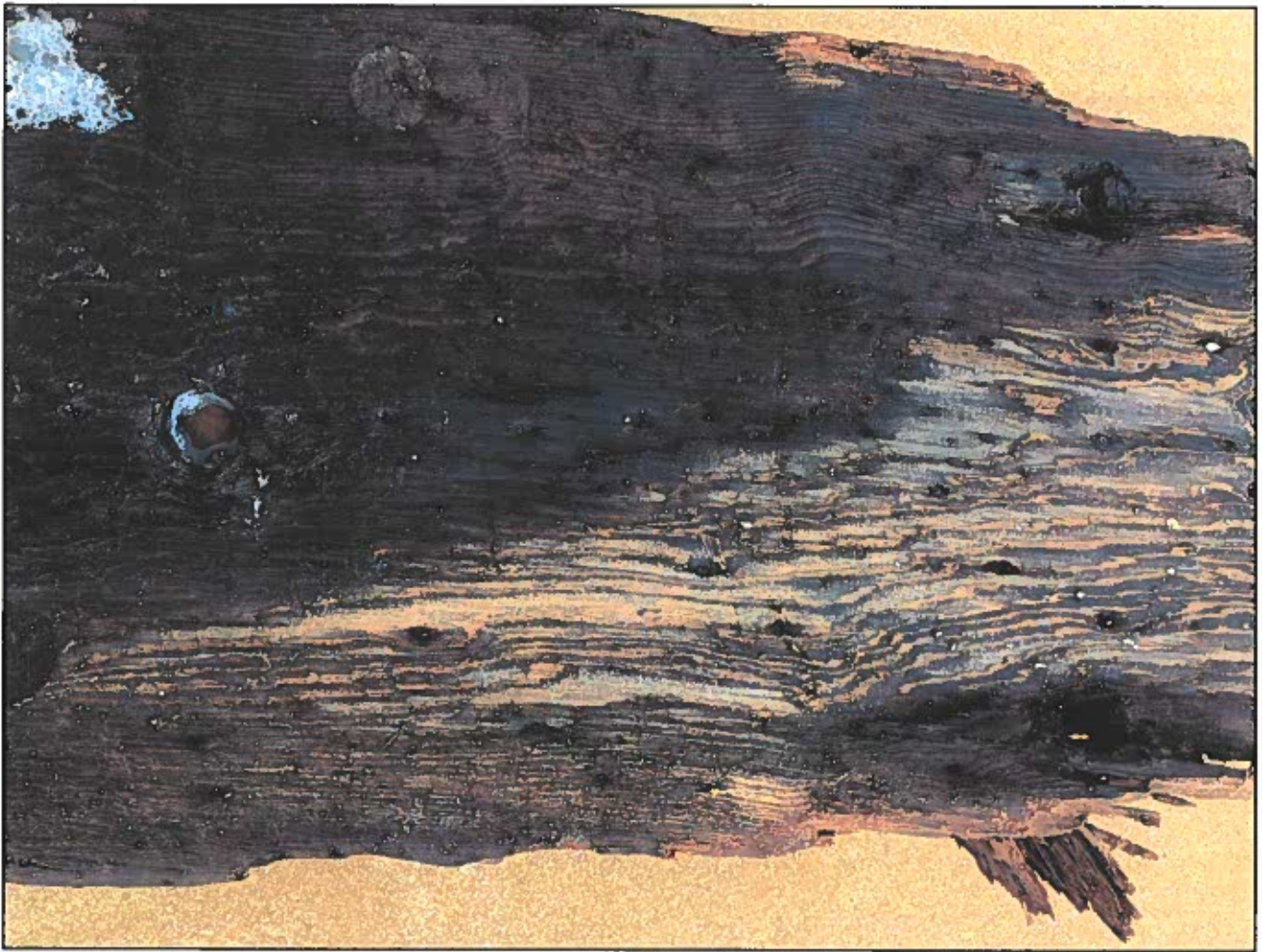
Sheathing tack holes (above) and details of plank end (below) (S. Langley Jan. 29, 2014).
