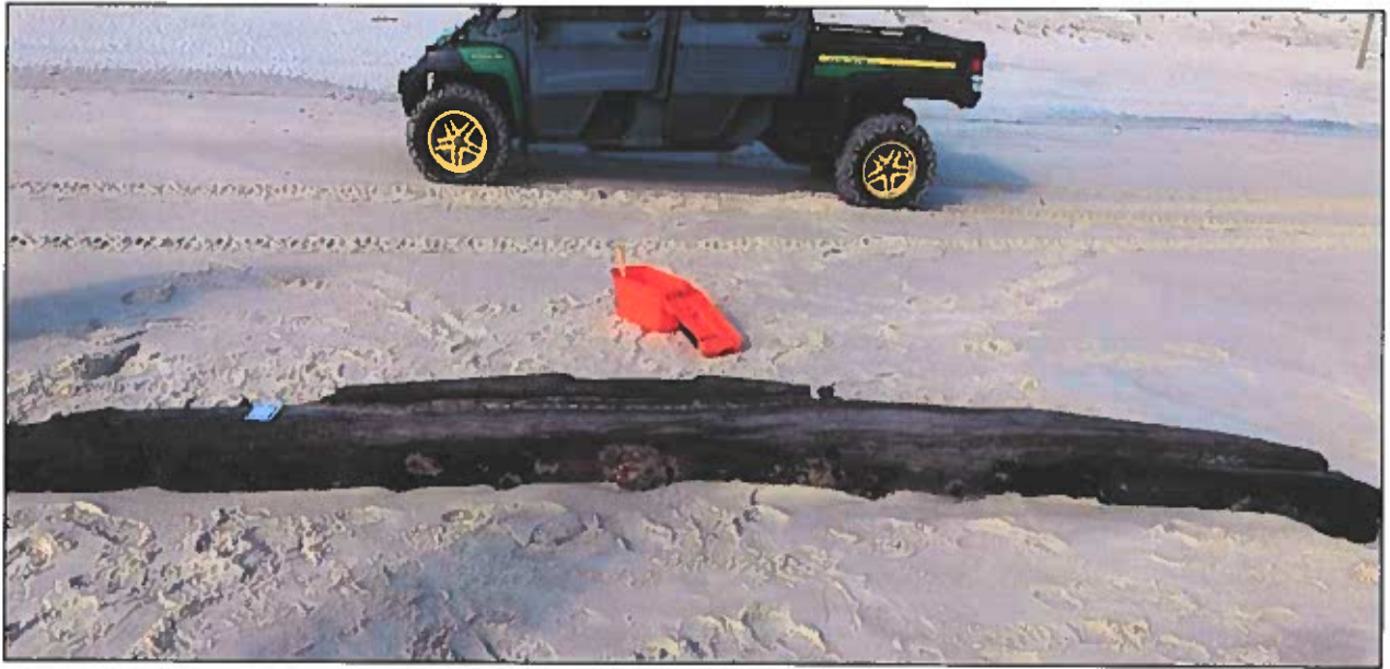
Keel notch attached separately (top center). Base of first futtock scarphed to floor timber (below). The floor and futtocks combine to make the ship's frames or "ribs."
