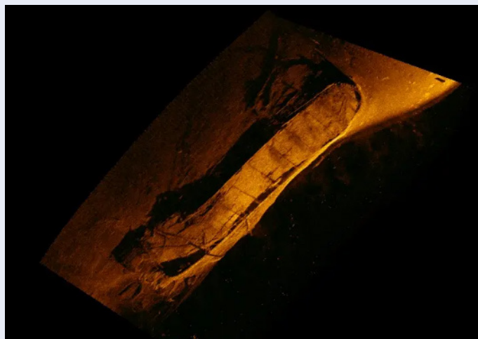
Side Scan Sonar Image of a Canal Boat on the Susquehanna River
