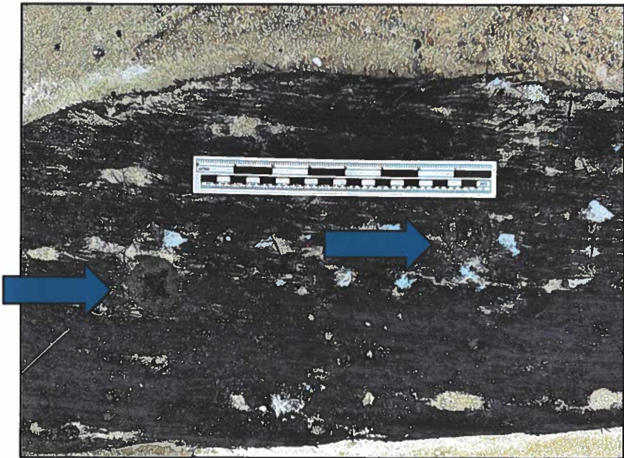
These machine-turned treenails appear to have the less common square shims.
